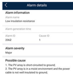
Figure E-1 Alarm details
